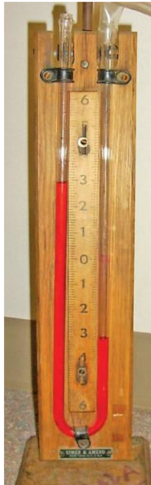
FIGURE 1–54 A simple U-tube manometer, with high pressure applied to the right side.
